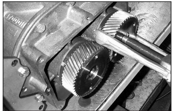
Figure 2. Pulling Driven Gear with Jaw Puller
